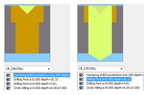
This is a quick way to verify the drilling operations generated for processing this part.
