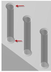
Attempting to machine these forms without easily splitting one of the chamfers to the opposite plane can be a time consuming task. ProDrill offers some intelligent strategies to machine such forms.
