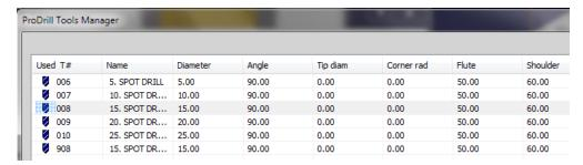
ProDrill highlight the 15mm spot drill. If you right click on the tool, the Mastercam Edit tool dialog is opened to allow you to edit the tool if needed. Otherwise, click on the tool as indicated below and click on OK to select the tool.
