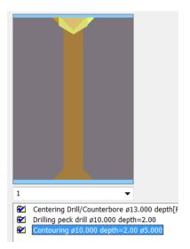
Delete the last 2 processes for peck drilling and contouring.
