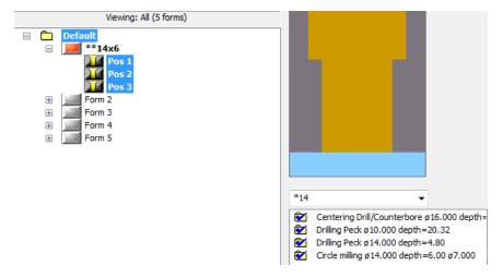
Lets apply a different process to Position 2 (Pos 2). In order to apply a separate process, lets create a cloned form for Pos 2.
