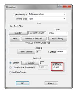
Click on **OK**. The resulting depth is now 80mm instead of 78mm. You will also note that the tool drills through the part.
