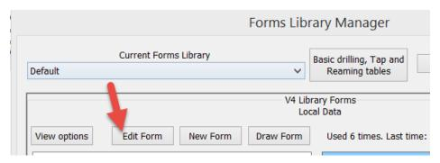
You can edit either any of the form's cylinders, modify the size, length, etc. and add additional cylinders if needed. You can also set any of the cylinders as reamed or tapped holes.
