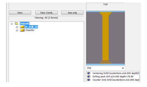
The second form that only has the chamfer has the Chamfer form applied with one operation.
