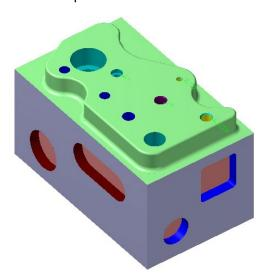
There are different cylinders marked with different colors for tapping and reaming. We have predefined color settings tables to determine the tapped and reamed sizes.
