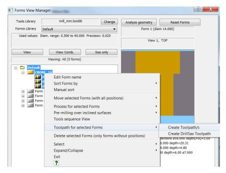
Mastercam toolpaths are automatically created for the selected form on the toolplane that the forms were identified on. In this case, it is the Top construction plane.
