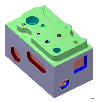
You can analyze the features if needed. You will notice that all the tapped forms were designed with the same color but ProDrill determines the tapped forms by scanning all the set colors with the internal diameters of the assigned tap table.
