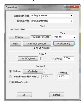
Click on **OK** to close the dialog. The following is the result for the list of operations. Note that the process name "**Copy-\*14**" now has a drilling cycle instead of an end milling cycle.
