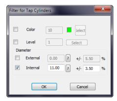
The cylinders that match the filtering options are highlighted in the graphics area. The menu also indicates the number of entities that match the filtered criteria. From the menu, click on "**Select All**". All 4 positions are selected and highlighted:
