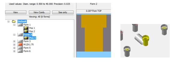
Add drilling processes by " **Apply Library (if it fails do Automatic)"** to "**Form 1**". A ream cycle is added automatically to the process.
