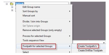
You will notice that the 2 drilling operations are done together. We do not want the counter sink operation (2nd operation) to be drilled for the bottom plane right after the centering for the top plane.
