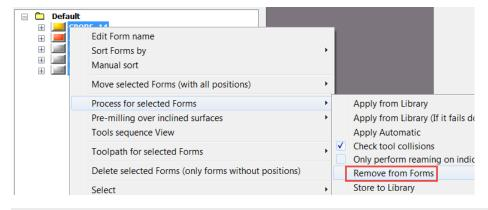
The part is now reset to the manner it was before applying processes to them. Now, apply a process again using the same menu and clicking on **Apply Automatic**.
