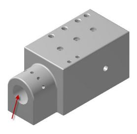
Since the other end of the selected cylinder is larger (80mm diameter) and previously machined no additional analysis is required.
