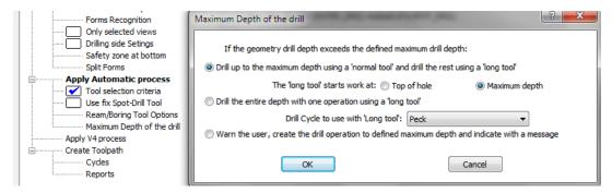
Leave the settings as shown above. The maximum depth value per diameter is set in the **A\_Drill** table of the automatic processes. You can access this table from the **Forms Manager.**
