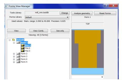
In the above case, we see that **Form 1** has 3 different positions. The image of Form 1, in this case a counter bored hole is displayed to the right of the form.
