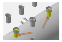
Click on **Do it** to set the forms as reamed forms. The reamed cylinders are identified by 360 degree yellow arcs at the top of the corresponding cylinder that needs to be reamed. The characters H7 are also written on top of the cylinder.
