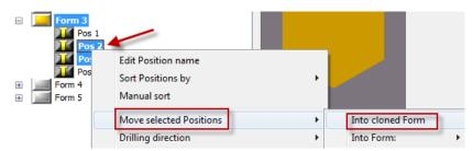
**Note**: Make sure the cursor is positioned close to the selected positions before right clicking. Click on "**Into cloned Form**". The 2 positions are now moved to a new Form group. The name of the group has the same name as the current form but with a suffix - **Cloned**. In this case, the name is "Form 3 - Cloned".
