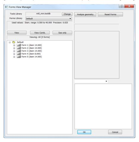
All the forms are identified on the part within the set diameter range. No toolpath operations are added to any of the forms. Clicking on any of the forms displays a graphics of the current form. **Highlighting a cylinder also displays the dimensions of the cylinder including the total depth at the corresponding cylinder**. When a Form is selected from the tree (in the case below, highlight Form1), the corresponding geometry is also highlighted.
