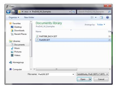
Select the file and click open . The drilling data that contains the reamed and tapped hole information is imported into Mastercam. All the holes that need to be reamed or tapped are marked with the corresponding red or yellow arcs in the appropriate drill form locations!
