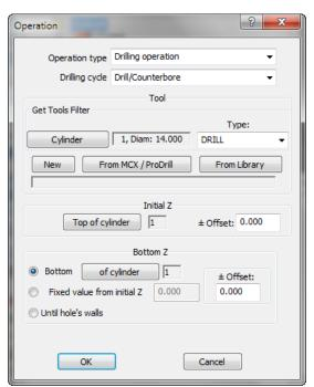
Using this dialog, we can define the first operation. The operation type and drilling cycle can remain the same. Choose a spot drill tool for this operation. The drill form diameter is 11mm. Click on **From Library** and choose a **Spot Drill** tool of **15mm** from the Tool library.
