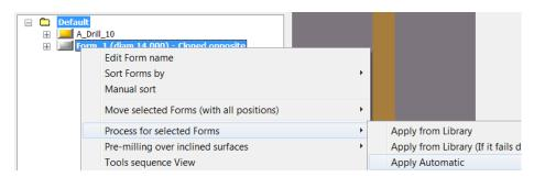
A new process is now added to the form. Note that in this case, all 3 drilling operations are added. To machine the chamfer, we only need a counter sink operation.
