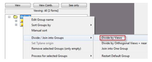
The result is 2 new groups according to the construction plane that the forms are identified on:
