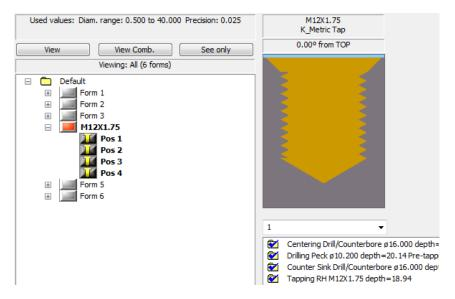
A safety depth for the tapping cycle is automatically applied from the tap library. Notice the drilling depth is calculated to 20.14 mm and the tapping depth to a lower value.
