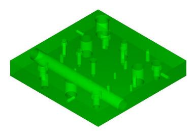
In order to mark the reamed and tapped forms, there is a drill feature data file that was generated using the Macro provided for SOLIDWORKS by ProDrill (review the Powerpoint presentation on using the Macro and generating the output file). This file has an extension .SDT that is normally stored with the same name and location as the SLDPRT file.
