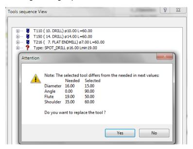
ProDrill intelligently verifies every step of the process definition and tool selection process to ensure that the right tool with the diameter and length are chosen to accomplish the task!
