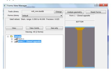
The following drilling processes are applied to Form 1. Upon simulating by selecting the drilling operation, you will notice that the drill depth is set to 78mm.
