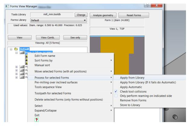
ProDrill searches for the drilling process in the new V5 Library. If it does not exist, it will prompt the user to use the Automatic Forms Process Manager (from Version 3) to create the drilling processes.
