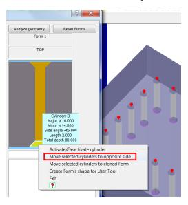
All the chamfers from the form are now moved to the opposite side. Note that ProDrill will not modify the actual geometry of the part in the process.
