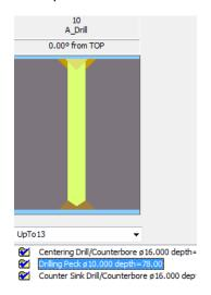
The depth is not sufficient to drill through the part if we are only going to apply the counter sink operation to the bottom side. We need to add an additional depth of 2 or 3mm to the process. Right click on the drilling operation and choose **Edit Operation**. For the Bottom Z depth, add a value of **-2mm** to the **offset** value.
