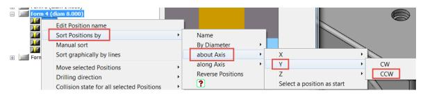
The positions are sorted about the Y axis in a counter clockwise direction and the result is as follows:
