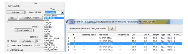
The following is the display after the tool selection. Now, you can set the spot drill depth. You can set this value as a fixed depth value. To do that, click on the "Fixed value from initial Z" and enter the value of **-1mm**. Make sure you set a negative value!
