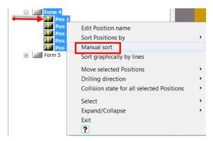
**Note**: The selection method is important. If you click on Form 4, all the forms will be added to the Layout Dialog. **You have to ensure that you right click when the cursor is on top of Pos 1!**
