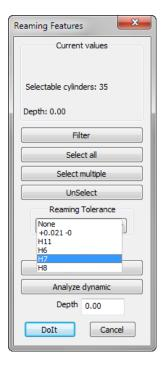
We will set the lower cylinders of 2 counter bored forms as H7 reamed holes. Click on the following cylinders. They will be highlighted as shown:
