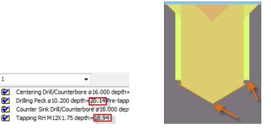
Upon doing a graphical tool use (by clicking on the different drill cycles), you notice the above - the tap tool stops at a safety distance.
