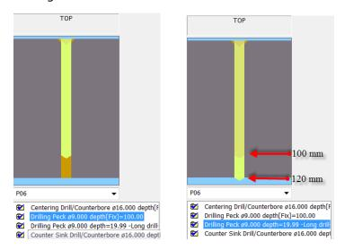
Creating the toolpaths will generate the corresponding drilling operations.
