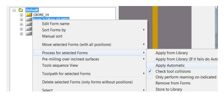
The following drilling processes are added. Note that the drilling processes are split into 2 operations. One operation that drills to a maximum fixed depth of 100mm and another that drills to the remaining depth.
