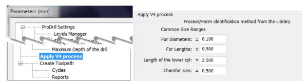
Setting a large value for the length of the lower cylinder can allow for most forms of similar types but varying minor diameter length to use the same process. If the value is small, ProDrill will prompt you with processes that match the form identified!
