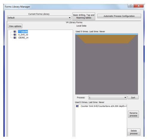
Let us **rename** the name of the form **\*\*10x90 to Chamfer.** Right click on the **\*\***10x90 and select **Edit Form name**. The name is highlighted for editing. Enter the new name.
